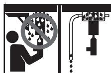
When carrying out "over" head wet cut core drilling, a water collecting ring and water suction are **always** to be used. These must be in perfect condition.
