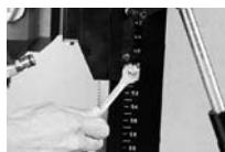
When using a drill stand a right setting of the guide block is required. Guide blocks for Rodia core drilling machines features slide strips for fine tuning on the drill stand.
